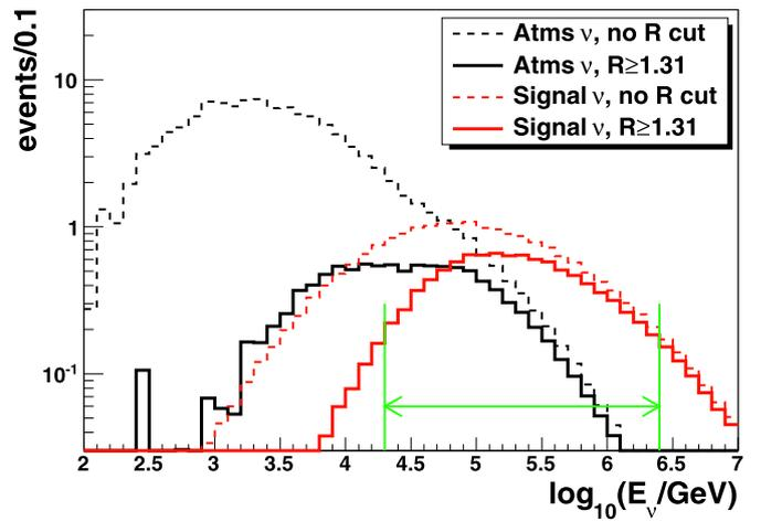
Fig. 4. Signal and background neutrino energy spectra as a function of the true neutrino energy after the second-level cut with and without the requirement  $R \geq 1.31$ . The energy region containing 90% of the astrophysical neutrino signal is indicated.
