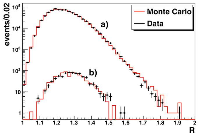
Fig. 2. Distributions of the number of events as a function of the  $R$  energy estimator for data and MC before the second-level cut. a) downgoing muons; b) mis-reconstructed as upgoing muons. The points are 12 line data, the histograms show the atmospheric muon MC normalized to the data.
