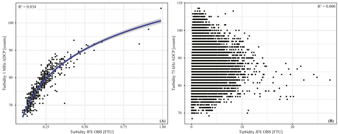
**Fig. 6.** Relation between recorded turbidity by the JFE Advantech OBS (x-axis) and the ADCPs (y-axis). A) Relation between JFE OBS and the Nortek 1 MHz ADCP; B) Relation between JFE OBS and the RDI Workhorse 75 kHz ADCP.
