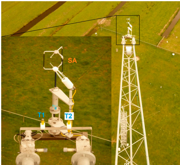
FIG. 3. Photos of the two downward-pointing NIOZ4 T sensors T1 and T2 mounted close to the sonic anemometer/thermometer SA at 60 m above ground on the tip of the SE boom, during the test experiment between 18 Apr and 5 Jul 2017.
