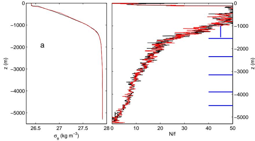
*Fig.4. Density and 40 m smoothed stratification with depth measured during LOCO-IW03. In the right panel horizontal lines indicate proposed current meter locations; vertical line shows the extent of the 75 kHz ADCP.*
