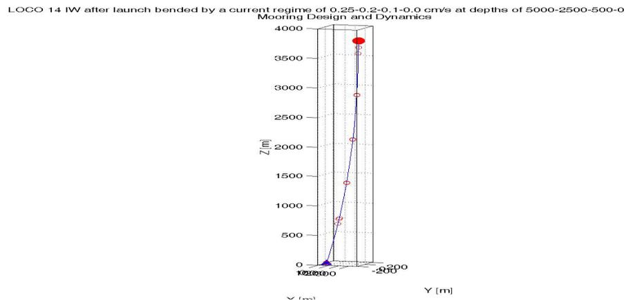
Fig. 3 Mooring deflection as computed by T. Hillebrand using program package designed by R. Dewey (UVic, Canada).
