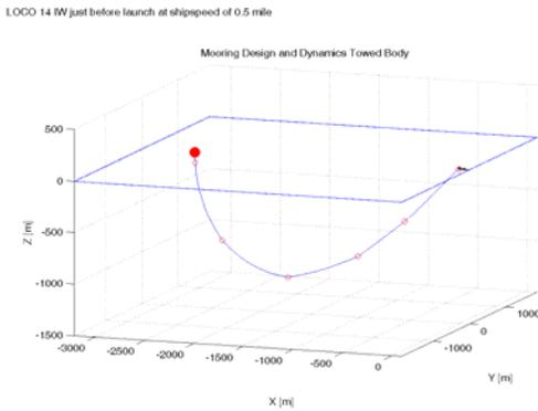
Fig. 10. Estimated mooring line at moment of release of anchor (computed by T. Hillebrand using program by R. Dewey, Uvic Canada).
