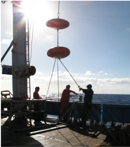
*Photo (P. van Breevoort): Elliptically shaped buoys in the mooring line.*
