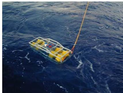
*Photo (M. Hiehle): Deep-towed body with two ADCP's.*
