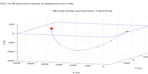
Fig. 5. Estimated mooring line at moment of release of anchor (acc. progr. R. Dewey, Uvic Canada).
