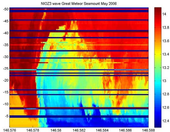
Fig. 9. Nearly 17 minutes of NIOZ-3 data in 50 m above the bottom, showing passage of large overturning wave in. The horizontal lines are partially bad sensors and partially poor calibration (that needs further treatment using a second calibration).
