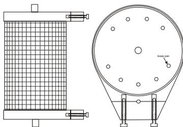
**Fig. 7.** Contaminant Sampler cage: sideview (left) and view from above/below (right).
