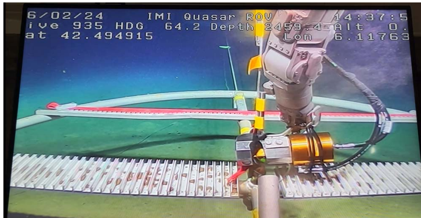
Figure 9. ROV-video screen image at the moment of cutting of a vertical line.
