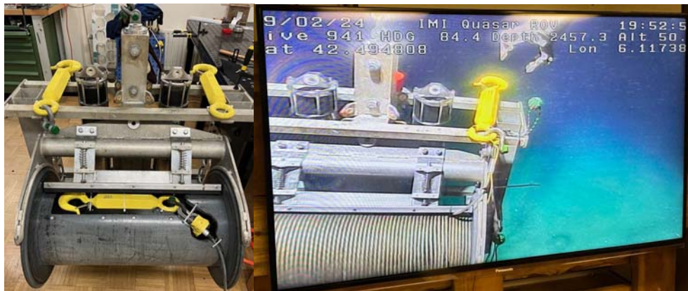
Figure 6. Frame with acoustic releases, drum to hold the 140-m steel cable with friction strip to avoid self-unrolling. One of 3 hooks to attach to cables is mounted inside the drum hold. The transponder beacon (red cap) is visible behind the acoustic releases (right image).
