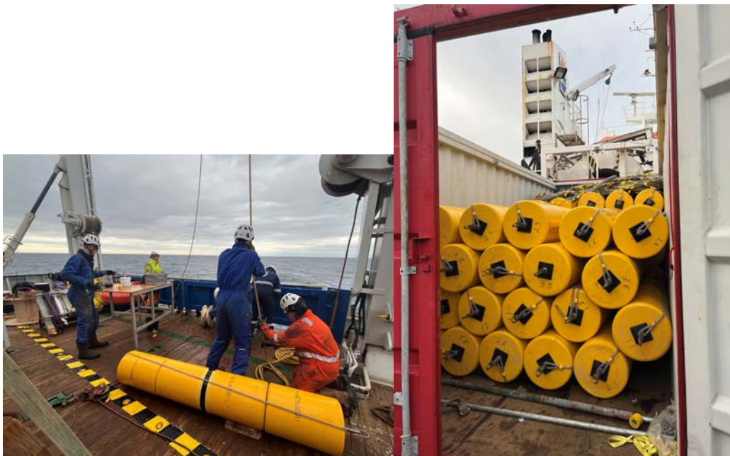
Figure 11. (left) Float hoisted on deck, spooling of line and grey case ready on the table to host the T-sensors to be cut from the mooring line. (right) Open-top container loaded with floats and mooring cables towards the end of the Phase-1 sea-operation.
