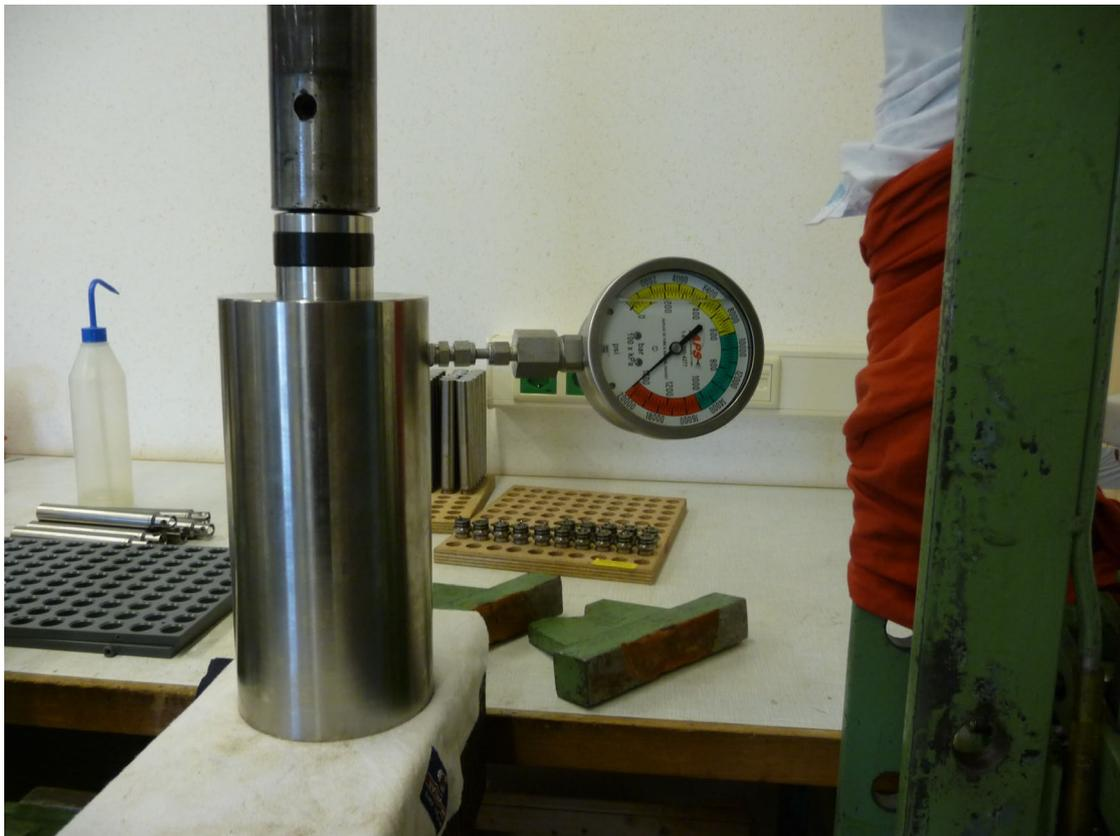
**Figure 2.** Custom-made titanium pressure container to test 7 high-resolution temperature sensors at 1400 Bar by applying about 40 Tons for at least 4 hours.
