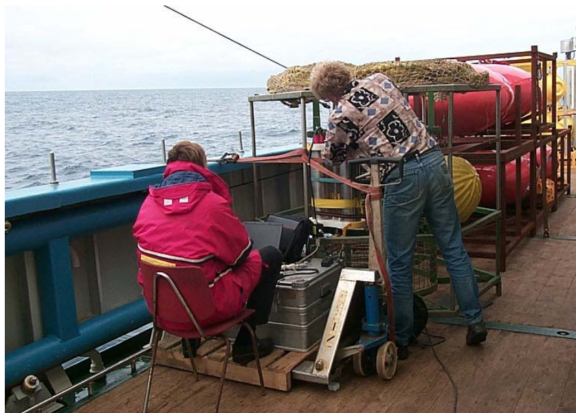
Fig 5. Spare CTD-frame holding NIOZ-thermistor strings for calibration (photo: Margriet Hiehle).
