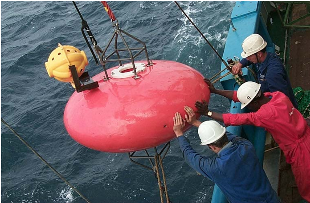
Fig4. Recovery of mooring ROCS-1 showing ellipsoidal buoyancy element with ARGOS beacon in yellow sphere (photo: Margriet Hiehle).
