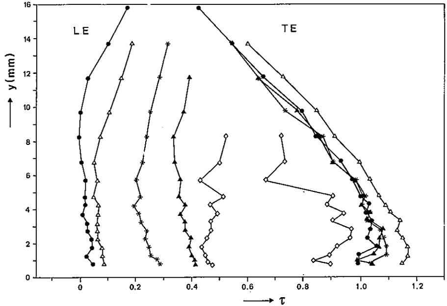
Fig. 4. The turbulent spot-edges in the  $y$ - $\tau$  plane.  $U_0 = 8.35$  m/s,  $x = 0.85$  m.  $\bullet$ :  $z = 0$  mm,  $\Delta$ :  $z = 15$  mm,  $*$ :  $z = 30$  mm,  $\blacktriangle$ :  $z = 45$  mm,  $\diamond$ :  $z = 60$  mm.
