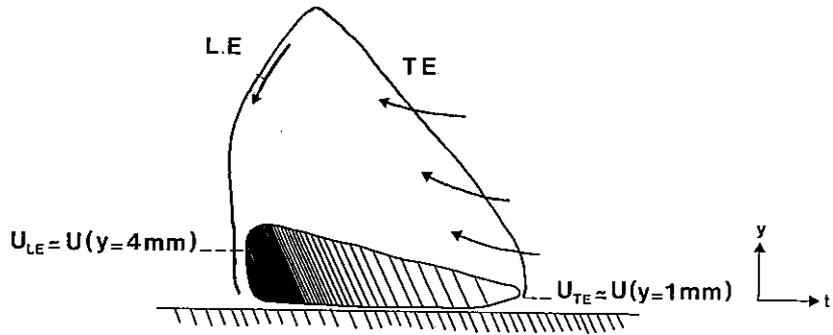
Fig. 11. Structure of the turbulent spot. Arrows indicate in- and outflow through TE and LE respectively. The shaded area represents the high turbulence intensity core of the spot.
