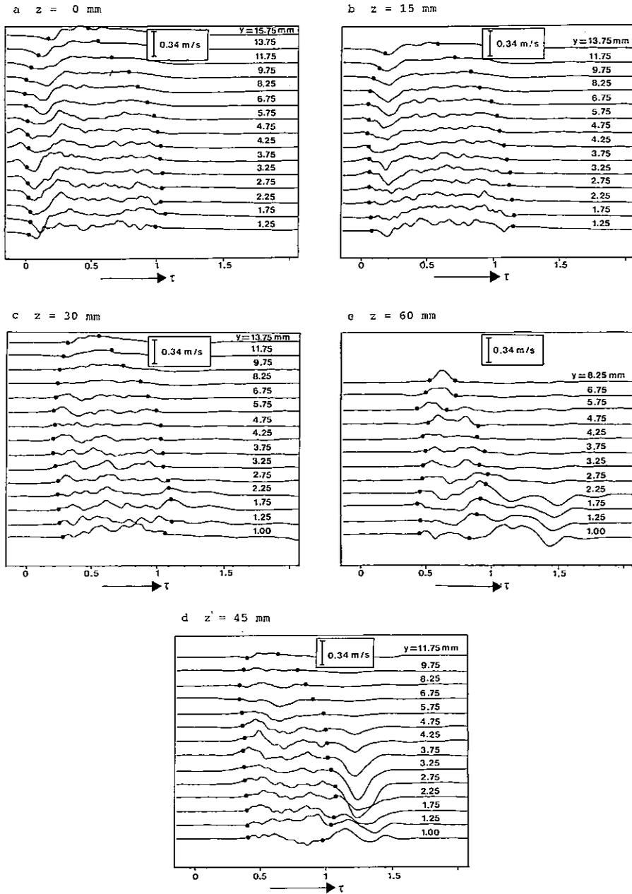
Fig. 7. The ensemble averaged  $\langle V \rangle$ -velocity distribution at the position  $x = 0.85\text{ m}$ ,  $U_0 = 8.35\text{ m/s}$ , for different heights  $y$ . The vertical bar indicates the  $\langle V \rangle$ -scale; the undisturbed lines in front of the spot indicate the  $\langle V \rangle = 0$  level for each height. a:  $z = 0\text{ mm}$ , b:  $z = 15\text{ mm}$ , c:  $z = 30\text{ mm}$ , d:  $z = 45\text{ mm}$ , e:  $z = 60\text{ mm}$ .
