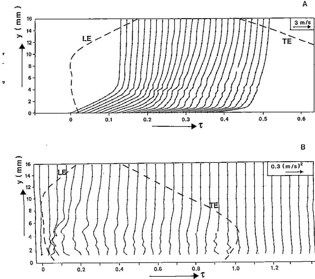
Fig. 10.  $\langle U \rangle$ -velocity profiles (10.a) and  $\langle uv \rangle$ -stress profiles (10.b) at  $x = 0.85\text{ m}$ ,  $z = 0\text{ mm}$ ,  $U_0 = 8.35\text{ m/s}$ . Dashed lines indicate LE or TE, reproduced from Fig. 4.
