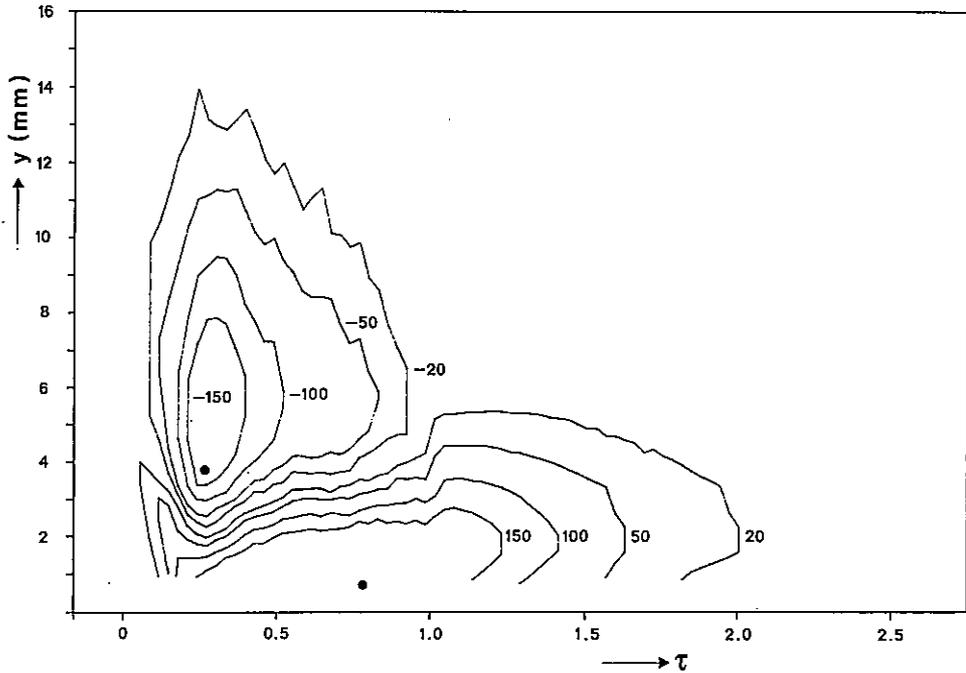
Fig. 9.  $\langle U \rangle$ -isotachs (in cm/s) at  $x = 85$  m,  $z = 0$  m,  $U_0 = 8.35$  m/s. The circles indicate the minimum ( $-200$  cm/s) and maximum ( $300$  cm/s) values.
