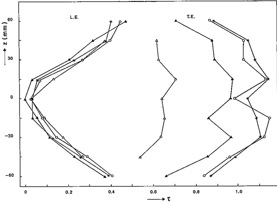
Fig. 5. The turbulent spot-edge in the  $z$ - $\tau$  plane.  $U_0 = 8.35$  m/s,  $x = 0.85$  m.  $\circ$ :  $y = 0.86$  mm,  $*$ : 1.75 mm,  $\blacktriangle$ :  $y = 6.75$  mm,  $\triangle$ :  $y = 11.75$  mm.
