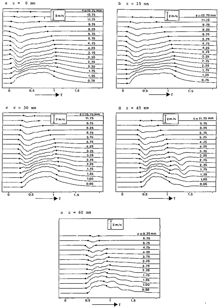
Fig. 6. The ensemble-averaged  $U$ -excess-velocity distribution at the position  $x = 0.85$  m,  $U_0 = 8.35$  m/s for different heights  $y$ . The vertical bar indicates the  $\langle U \rangle$ -scale; the undisturbed lines in front of the spot indicate the  $\langle U \rangle = 0$  level for each height. a:  $z = 0$  mm, b:  $z = 15$  mm, c:  $z = 30$  mm, d:  $z = 45$  mm, e:  $z = 60$  mm.
