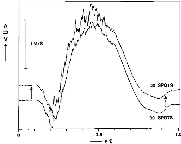
Fig. 3. The influence of the number of spot realisations on the ensemble average (origin translated as indicated by arrows).  $U_0 = 8.35$  m/s,  $x = 0.70$  m,  $y = 2.0$  mm and  $z = 0$  mm.
