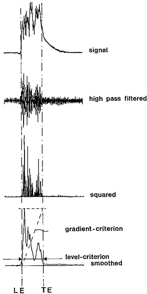
Fig. 2. Detection scheme for the determination of spot leading and trailing edge as applied to the  $U$ -velocity-signal.
