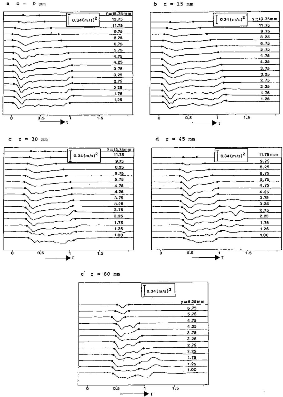
Fig. 8. The ensemble averaged  $\langle uv \rangle$ -distribution at the position  $x = 0.85$  m,  $U_0 = 8.35$  m/s, for different heights  $y$ . The vertical bar indicates the  $\langle uv \rangle$ -scale; the undisturbed lines in front of the spot indicate the  $\langle uv \rangle = 0$  level for each height. a:  $z = 0$  mm, b:  $z = 15$  mm, c:  $z = 30$  mm, d:  $z = 45$  mm, e:  $z = 60$  mm.
