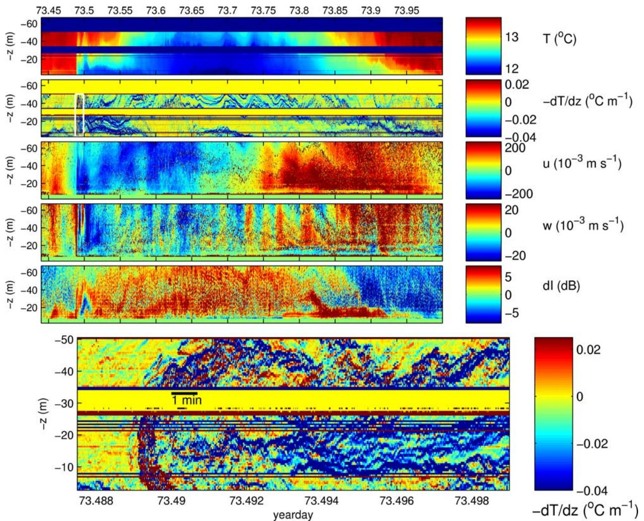
**Figure 2.** One tidal period of ADCP and thermistor string data. The white rectangle in temperature gradient ( $dT/dz$ ) indicates the lowest panel, which shows 20 minutes of data of a bore. Bad data in temperature ( $T$ ) or  $dT/dz$  are visible by coloured horizontal bars. A similar bar between 3–7 m indicates ‘no data’ in ADCP records (cross-slope  $u$ , bottom-normal  $w$  and relative backscatter  $dl$  corrected for water attenuation). Scattered bad data in the ADCP records are brown.
