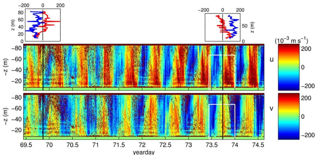
**Figure 1.** Entire depth-time series of ADCP data  $u$  (positive downslope) and  $v$  (positive  $\sim$ poleward). Two examples of bi-directional cross-slope flow (red) are shown in the upper panels with  $v$  (blue) at times marked by the black lines. The white rectangle indicates Figure 2.
