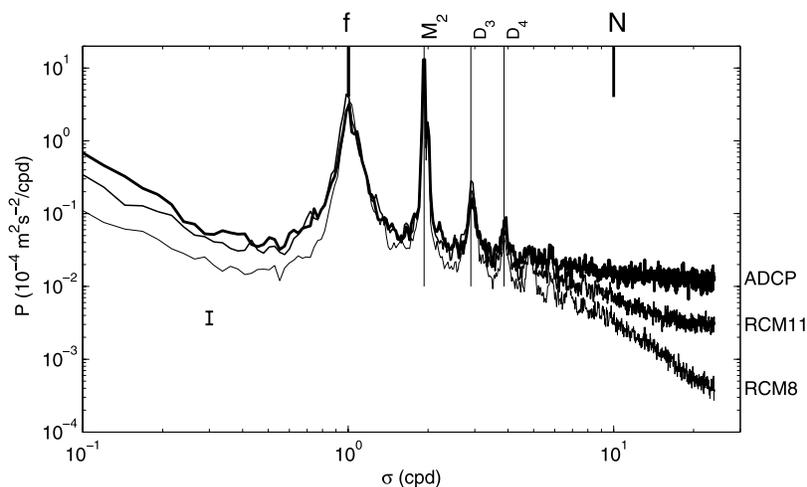
**Figure 2.** Spectral comparison of 1.5 years of Canary Basin data in a single mooring for acoustic devices (RDI-75 kHz ADCP, 1140 m, thick line; Aanderaa RCM11, 1460 m, medium line) with a mechanical Aanderaa RCM8 (2260 m, thin line).
