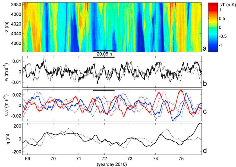
**Figure 3.** One week of deep internal wave observations. (a) Depth-temperature image relative to  $\Gamma$ . The inertial period is indicated. (b) Two-hourly smoothed vertical currents observed 2 m above uppermost T-sensor (solid) and 196 m below lowest (dashed). (c) Corresponding horizontal current components  $u$  (blue) and  $v$  (red). Note the scale increase compared to Figure 3b by a factor of 2. (d) Vertical excursions computed using (1) with  $w$  taken from Figure 3b.
