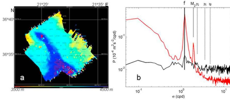
**Figure 1.** (a) Shipboard multibeam image obtained just prior to mooring launch (x) in northern part of trench. Colour coding for 3500 (red) to 4500 m (blue); red speckles near the bottom are errors. (b) Kinetic energy (red) and vertical current (black) spectra. Several frequencies are indicated: inertial frequency ( $f$ ) including several higher harmonics and semidiurnal lunar tidal ( $M_2$ ).
