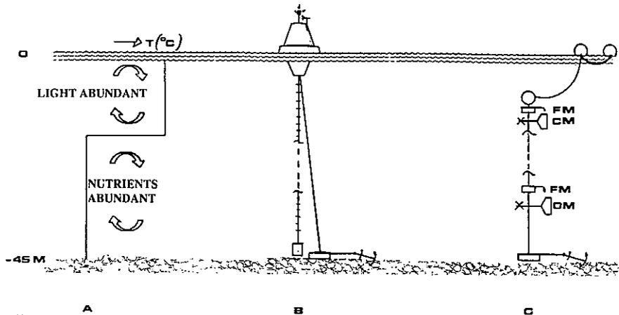
Figure 2. Schematic of the types of mooring used during INP and a sketch of the "classic" two-layer stratification, indicated by the temperature profile as a function of depth in A. B. Surface mooring with meteorological data buoy and thermistor strings. C. general mooring with current meters (CM) and fluorometers (FM).
